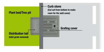
The pipe socket in the bottom part kan either be sealed or provided with a riser pipe that connects to a well. The riser pipe is used as an overflow protection to prevent possible flooding in the plant bed. If the distribution tub is used on its own, Combi Plus should be installed in mortar to seal the pipe socket and stabilize the bottom part.
